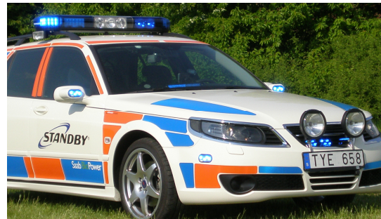
Six blue lamps mounted on a police car in the rear view mirrors, under the head lamp and above the license plate.
