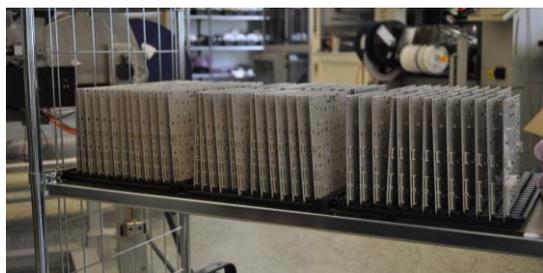
***Surface mounted LED modules at Aluwave production***
