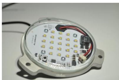
***LED-based light source made by Aluwave***
